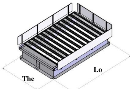
The range is able to open the ARCALAM EVOLUTION ELECTRIC despite the presence of an unfavorable wind of 10 m/s and an overload of: 25 kg/m<sup>2</sup> or 50 kg/m<sup>2</sup>.
