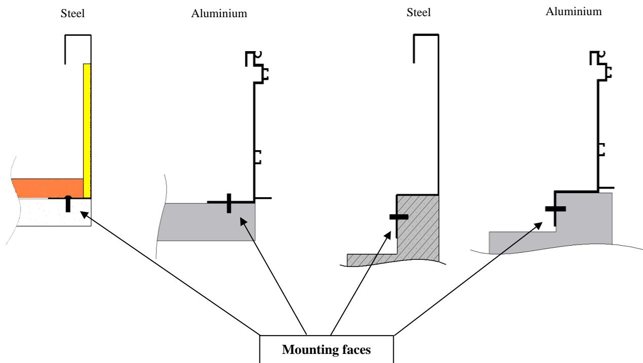
**Be careful, any other place for fixing, may cause water leaks.**
